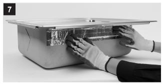
Keeping the SinkMate backing strip centered, completely cover the SinkMate backing strip with foil tape as shown. Do NOT leave any portion of the SinkMate backing strip exposed.
